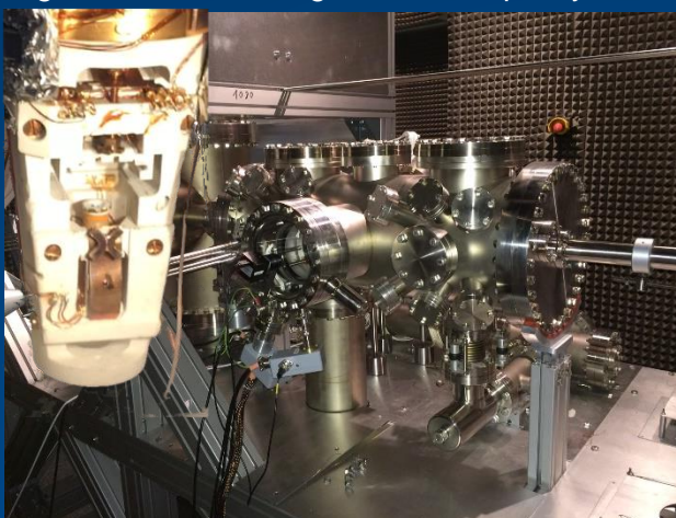
Fig. 2: The UHV-System with the new low temperature STM (inset) made from ceramics.
