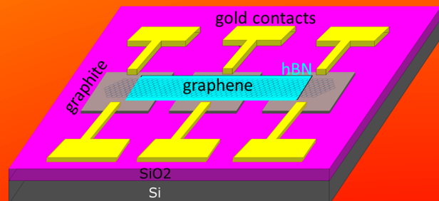
Fig. 1: Sketch of a typical graphene device
