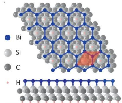
Fig. 1 Sketch of a two dimensional sheet of Bismuthene on a SiC(0001) substrate [1].
